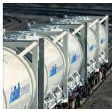
ISO-Veyor tank containers from InBulk Technologies are increasingly used for transporting cement
